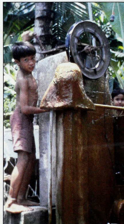
A rope pump, built and installed by Rus at a cost of only $5, is something even children can operate easily.
